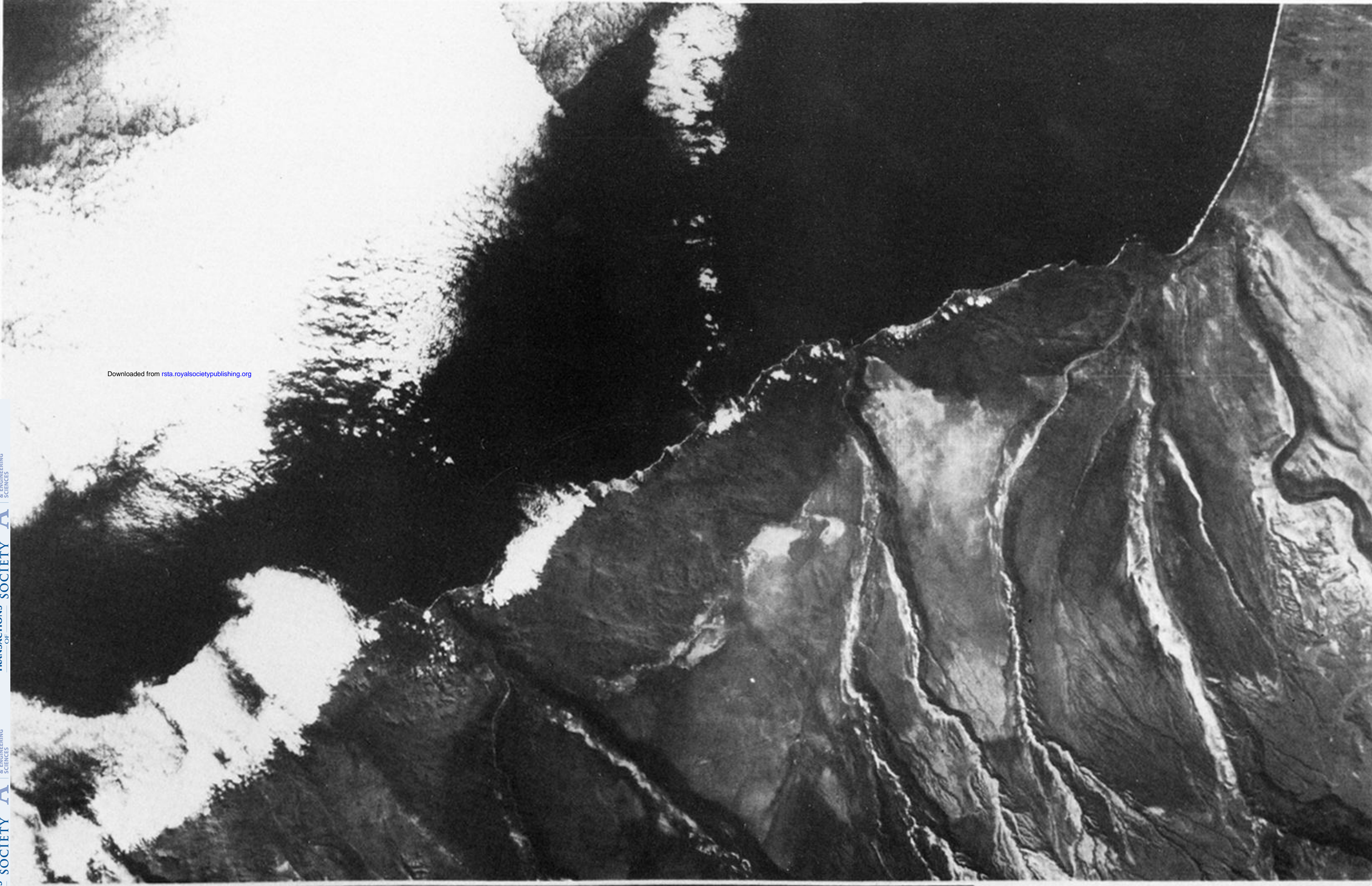
FIGURE 12. SPAS-MOMS imagery. This is the very first MOMS-1 picture (raw data). It shows the coast of Chile near Africa with the Andes. It is a full-scale picture (138 km \times 94 km) with approximately 4720 scan lines with 6912 pixels each. It was imaged during the STS-7 mission on 20 June 1983; the Sun elevation angle was 40.5^\circ . (Data pre-processing and image processing by M.B.B. and R. Haydn (University of Munich).)
